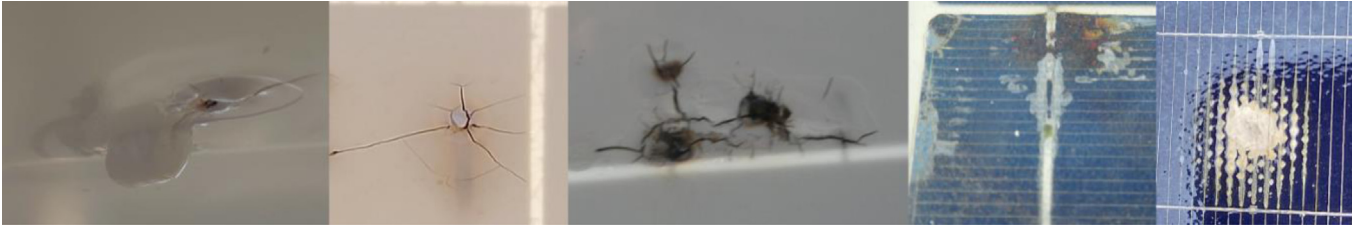
Fig. 1. Potential/observed consequences of (cyclic) shading: bubbles, blisters and burn marks.
