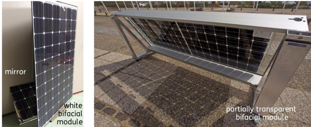
Fig. 2. Illustration of reflective mesh between solar cells in bifacial module. (left) Experimental bifacial module from ECN in 2016 [24] and (right) partially transparent, bifacial solar panel outdoors in the sun. Whereas in the white bifacial case, there is no light transmitted to the wall behind the panel, we can clearly see the ground irradiance distribution and shading pattern of the partially transparent bifacial module.
