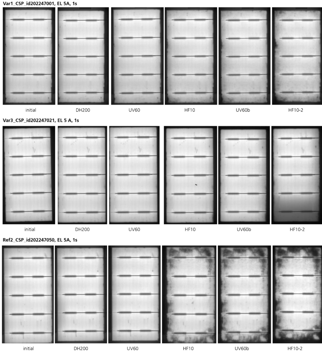
Fig. 8. Selected EL images to analyze the degradation during sequence B.
