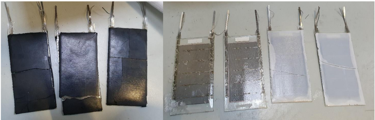
Fig. 7. Photos of specific samples after DH200: left) Var 4 (PLA), right) Var 6 samples with coating.
