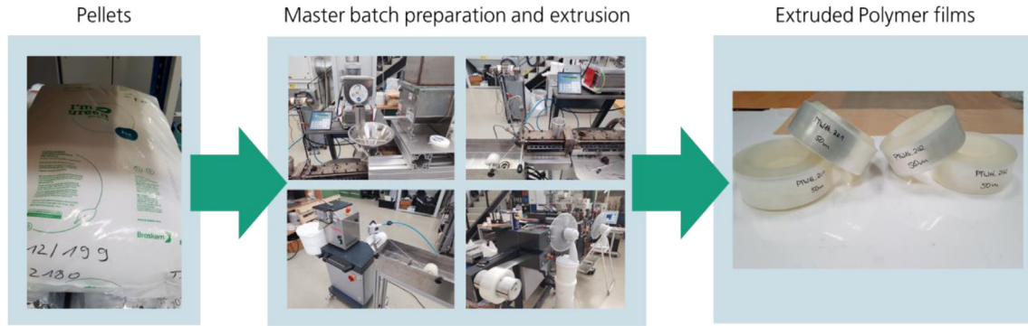
Fig. 1. Schematic overview of the customized in-house extrusion of EVA encapsulants at the Fraunhofer IMWS.
