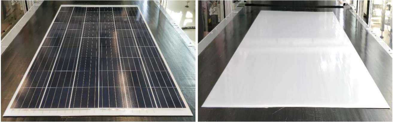
Fig. 17. 60 cells GB PERC module laminated for process optimization, front side (left) and rear side (right).
