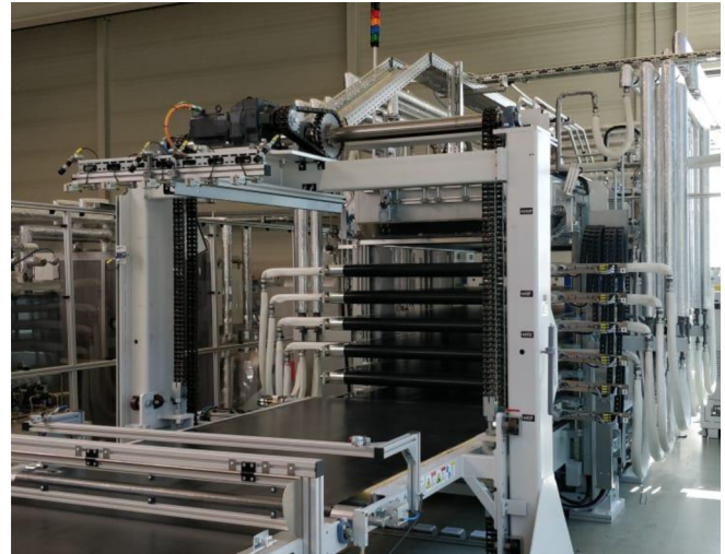
Fig. 5. Lab Laminator used for gel content sample preparation and process optimization at Buerkle.
