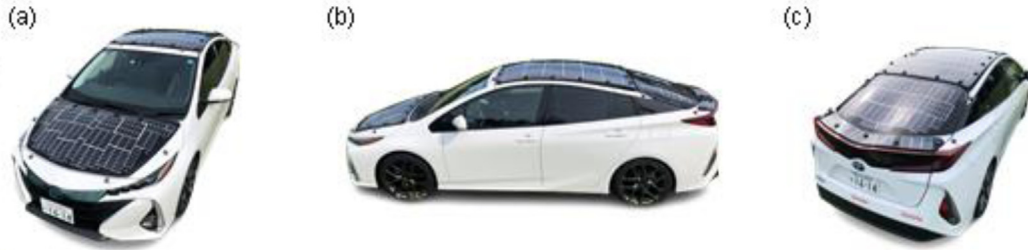
Fig. 1. Photographs of the solar-powered car equipped with III-V triple-junction PV modules.
