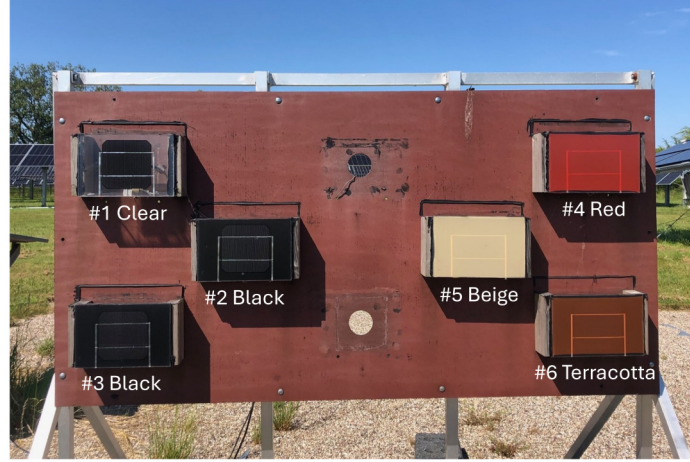
Fig. 1. The mini-module setup at Risø, including one clear, two black, one red, one beige, and one terracotta single-cell glass-glass module. This picture was taken in the period when all mini-modules operated in a ventilated condition.
