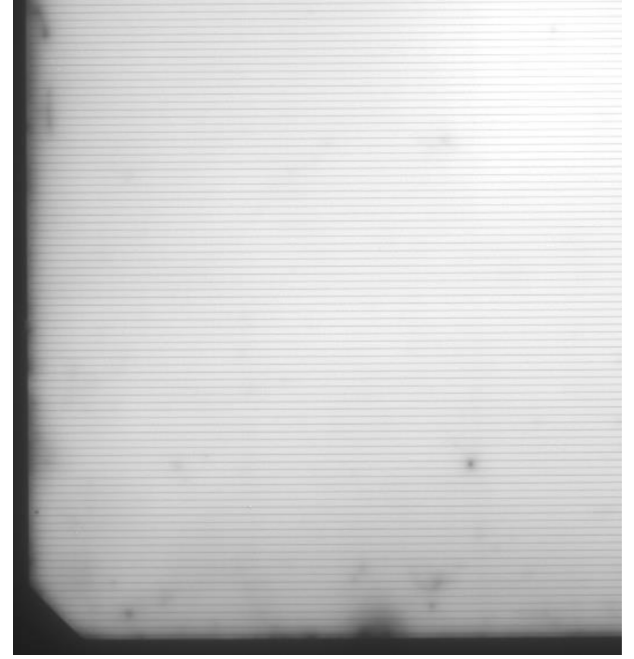
Fig. 6. Zoomed view of one corner of an exemplary photoluminescence image of SelFi TOPCon cell from G6 with the p + poly-Si fingers visible as darker horizontal lines.
